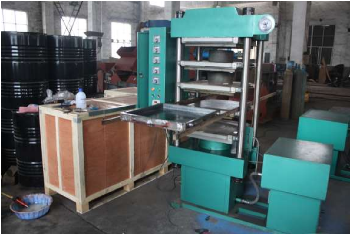
Compression molding equipment at vendor factory in Shanghai ready for shipment.
